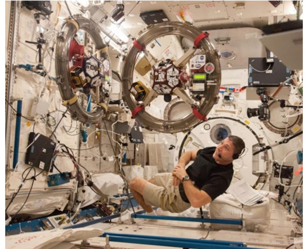
Rings is a electromagnetic based propulsion system run by MIT Space Systems Laboratory. The experiment utilizes 2 SPHERES vehicles that are places inside the RINGS support structure and interfaced together through the SPHERES expansion port via a ribbon cable. (NASA)
